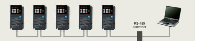
Multi-drop connection possible at terminals Compatible with Modbus communication
