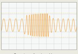
Current waveform in sudden acceleration/deceleration at 0.5Hz
