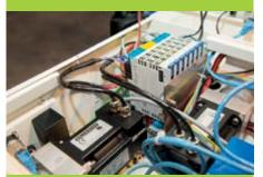
Even in the confined interior of the AGV PackMan 200, there is space for the vibration-proof S-DIAS system with motion control and Safety, as well as two AKM low-voltage DC servo motors.
